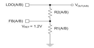
Figure 2: Selection of External Resistors.
