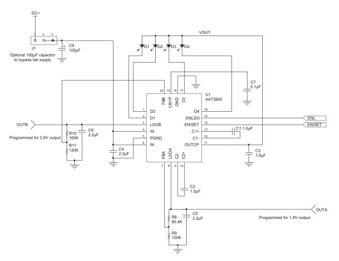
Figure 5: AAT2845-EE Section Schematic.
