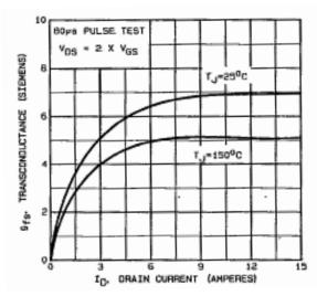
Fig. 11 - Typical Transconductance vs. Drain Current
