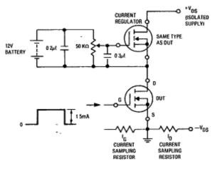
Fig. 17 - Gate Charge Test Circuit
