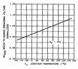
Fig. 12 - Breakdown Voltage vs. Temperature
