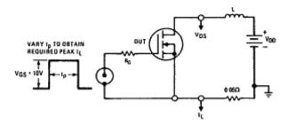
Fig. 15a - Unclamped Inductive Test Circuit
