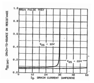
Fig. 13 - Typical on-Resistance vs. Drain Current
