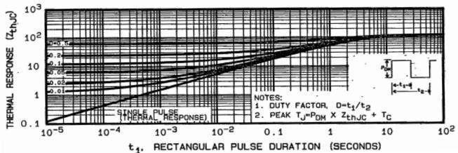
Fig. 10 - Maximum Effective Transient Thermal Impedance, Junction-to-Ambient
