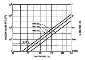
Fig. 18 - Typical Time to Accumulated 1 % Gate Failure
