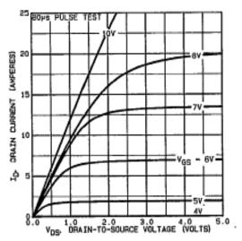
Fig. 2 - Typical Output Characteristics
