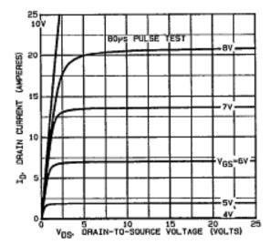
Fig. 1 - Typical Output Characteristics
