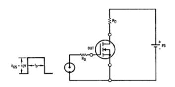
Fig. 16 - Switching Time Test Circuit
