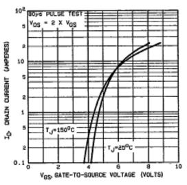
Fig. 3 - Typical Transfer Characteristics
