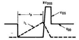
Fig. 15a - Unclamped Inductive Load Test Waveforms
