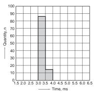
7.-(1) Electrical life test (at resistive load) Sample: CP1-12V Quantity: n = 4 (N.C. = 2, N.O. = 2) Load: Resistive load (N.C. side: 10A 14V DC, N.O. side: 20A 14V DC)
