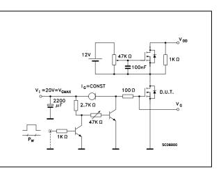
Figure 14. Gate charge test circuit
