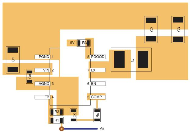
Figure 3. AOZ1020A (SO-8) PCB Layout
