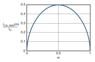
Figure 2. I<sub>CIN</sub> vs. Voltage Conversion Ratio
