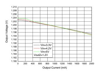
OUT2 Line Regulation vs. Input Voltage
