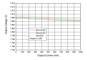
OUT1 Line Regulation vs. Input Voltage
