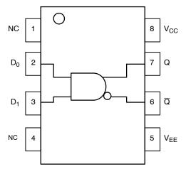
Figure 1. Logic Diagram and Pinout
