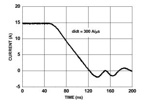
Figure 13. SyncFET body diode reverse recovery characteristic
