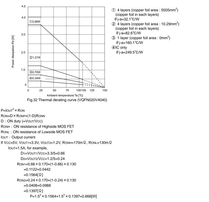
As RONH is greater than RONL in this IC, the dissipation increases as the ON duty becomes greater. With the consideration on the dissipation as above, thermal design must be carried out with sufficient margin allowed.
