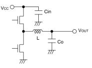
Fig.35 Input capacitor
