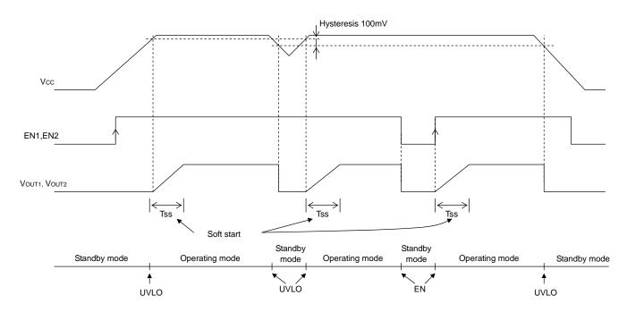
Fig.30 Soft start, Shutdown, UVLO timing chart
