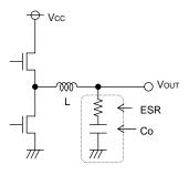
Fig.34 Output capacitor
