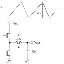
Fig.33 Output ripple current
