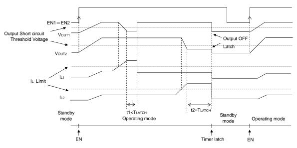
Fig.31 Short-current protection circuit with time delay timing chart
