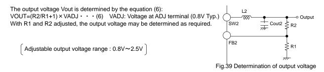
Use 1 k $\Omega$ ~100 k $\Omega$  resistor for R1. If a resistor of the resistance higher than 100 k $\Omega$  is used, check the assembled set carefully for ripple voltage etc.
